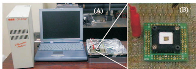
Figure 1. Schematic photograph of the CV50W and micor-device set-up system for the detection of L-lactate.
